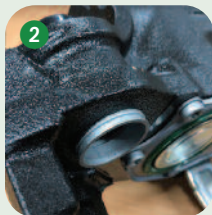
The relieved casting and extended metal ring for fitment of a sealing boot
